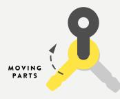
Snap the heads of connectors into the groove of another to create a fully rotating joint. Push the leg all the way through to create a joint with limited movement.
