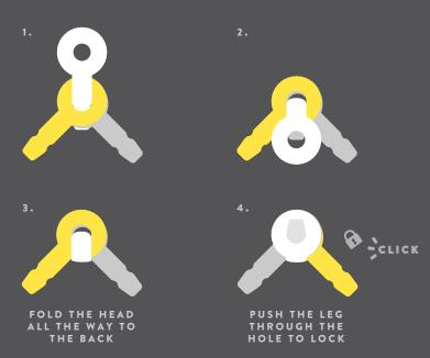
With the moving joint fold the head over to the other side and snap it into the groove to create a friction lock. The legs will shift and hold in different positions.
