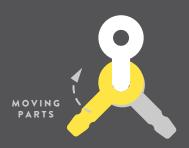
Snap the heads of connectors into the groove of another to create a fully rotating joint.
