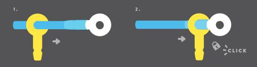
Snap onto the groove.
