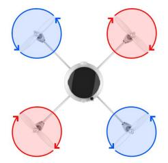
One set of propellers has a negative angular momentum and the other set have a positive angular momentum. However, the net angular momentum at the drone body is zero.
