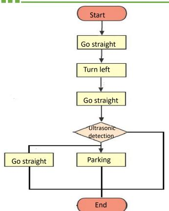
By keeping the parking route in the mind, design a flow chart of Q-scout parking onto the designated space, analyse and try your skill of programming logics for the challange.
