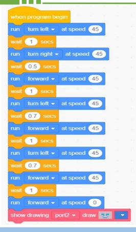
Programming on the basis of Captain Alloy's route, in actual operation, it can debug the time of advancing and turning according to different fields.
