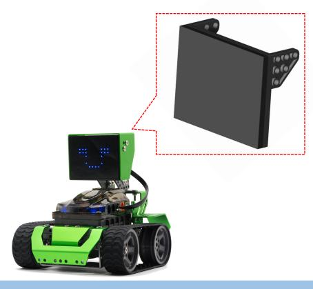
LED matrix screen consists of 140 LED lights, according to signal, LED light on matrix screen will shining or not shining when use connection line to connect mainboard and the port of LED matrix screen, and it will appear pattern that you want obeying changes of command.
