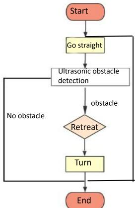
3. As per the flowchart, the program of Q-scout has been written to avoid the obstacles on a difficult terrain. Did you check whether it is working well or not.
