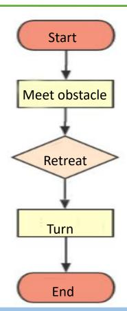
When Q-scout detects an obstacle in front of it, in order to avoid the obstacle better, Q-scout reverse for a certain distance before turning to avoid the obstacle.
