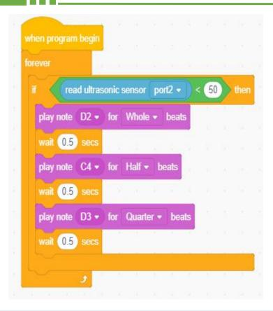
In the computer programming software, try to write Q-scout danger alarm program.
