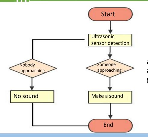
When the Q-scout detects someone approaching in front of it, the sensor sounds an alarm. If no one is approaching, no sound is generated.
