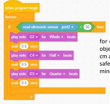
As per the flowchart designing, write a program for our Q-scout to sound a danger alarm when an object has reached to a specific distance (let's say 50 cm away from sensor). The alarm should be started at safe distance so that person can get enough time to mind his/her steps.
