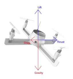
of two adjacent motors and increasing the speed of the other two motors by the same factor. For example, if you wish to move the drone to the right as pictured in the free body diagram above, the speed of the two motors on the left should be increased and the two motors on the right should be decreased.
