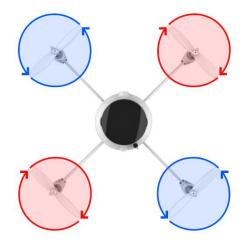
One set of propellers has a negative angular momentum and
