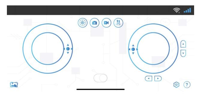
The left joystick changes the yaw and altitude of the drone (up/down). The right joystick changes the pitch and roll (right, left, forward, backwards).
