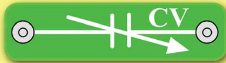
Variable Capacitor (CV)
